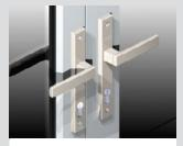
We offer 4-point lever compression locking as standard. This ensures high performance seals and improves air infiltration resistance. ICON™ stainless steel furniture shown above.
